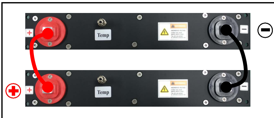
<Fig. 3> Parallel Connection of Modules.
