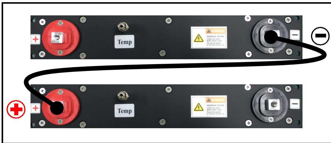
<Fig. 2> Series Connection of Modules
